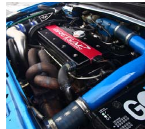
Below: Astra's 2-litre unit dishes out 420bhp, 183 more than standard. Bottom: Golf is up 210bhp to 407
